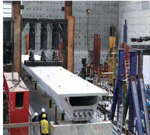
Static Loading Test of Ultra-High Performance Concrete (UHPC) Prestressed Simply Supported Beams (U258)
