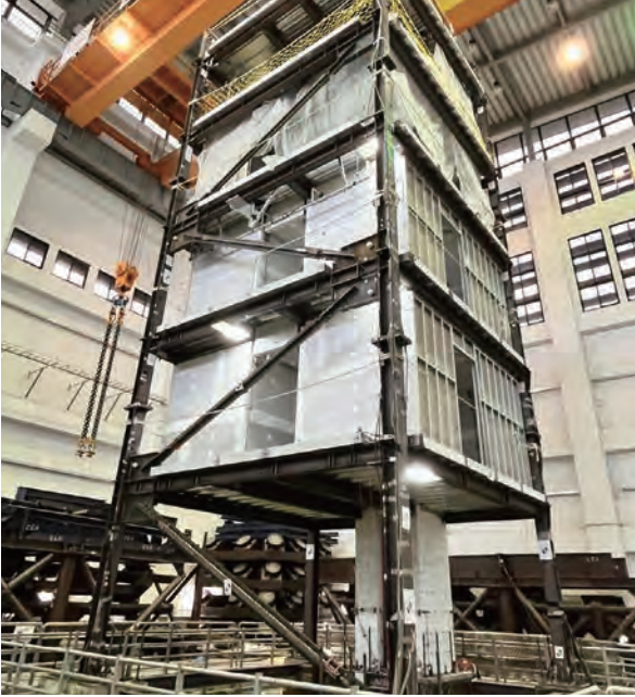
Exterior view of the test specimen developed in collaboration with New Zealand universities.
