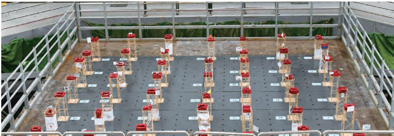
Models preparing to undergo testing after being mounted on the shaking table.
